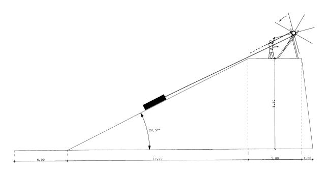
Fig. 12. Design of the winch at the top end of the ramp.
