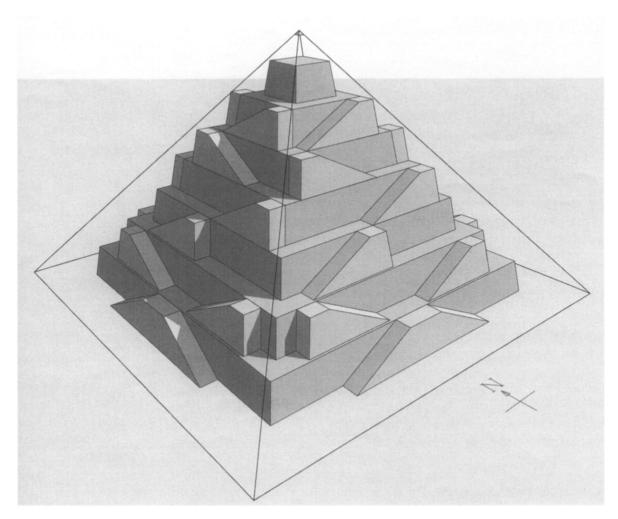
Fig. 11. Ramps used for construction of the stepped core (perspective drawing).
