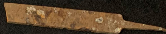
American Pattern Hand File Collins Homestead & Cotton Gin, Birdston Valley Community (Early to mid-20 th century) This file may have been used for sharpening cotton gin saws or farm tools.
