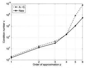
Fig. 3.4. Condition numbers of the quasi-stiffness matrices.
