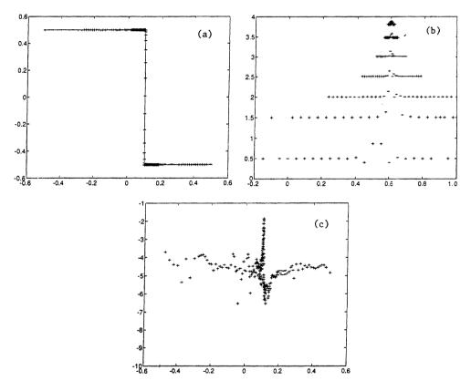
FIG. 12. Adaptive wavelet collocation solution of linear PDE (6.4) with initial condition (6.3) ( $\delta = 0.004$ ) at t = 0.1 with L = 20, J = 8, and error tolerance  $\epsilon = 10^{-4}$ . The number of collocation points N = 240. (a) plus sign—numerical solutions, solid line—exact solution; (b) wavelet coefficients at all levels; (c) errors at collocation points in logarithm scale.
