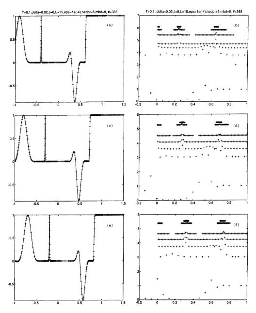
FIG. 13. Adaptive wavelet collocation solution of linear PDE (6.4) with initial condition (6.1) ( $\delta = 0.02$ ) at t = 0.1, 0.2, 0.3 with L = 15, J = 8, and error tolerance  $\epsilon = 10^{-4}$ . The number of collocation points N = 385, 394, and 392 at time t = 0.1, 0.2, and 0.3, respectively. (a)-(c) plus sign—numerical solutions, solid line—exact solution; (d)-(f) wavelet coefficients at all levels.
