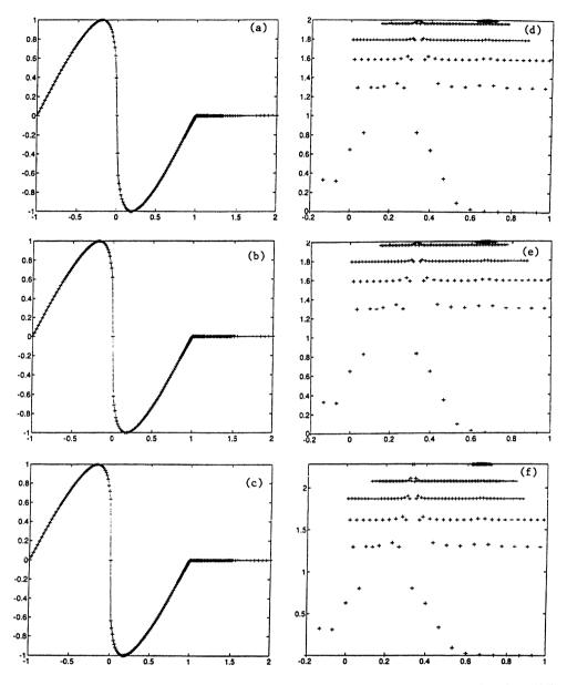
FIG. 14. Adaptive wavelet collocation solution of inviscid Burger's equation (6.5) with initial condition (6.6) at t = 0.3, 0.318, 0.319 with L = 15, J = 8, and error tolerance  $\epsilon = 10^{-4}$ . The number of collocation points N = 292, 295, and 303 at time t = 0.3, 0.318, and 0.319, respectively. (a)-(c) plus sign-numerical solutions; (d)-(f) wavelet coefficients at all levels.
