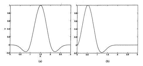
FIG. 2. Interior wavelet functions  $\psi(x)$  (a) and boundary wavelet function  $\psi_b(x)$ .
