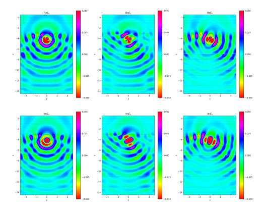
FIG. 4.1. Electric fields in a 10-layer medium described in section 4. Fields are computed along x = 0.2 for  $-5.0 \le y \le 5.0$  and  $-14.5 \le z \le 0.5$ . The contouring level is clamped to the range (-0.05, 0.05) for a clearer illustration of wave pattern and avoiding the peak values near the source, which is located in the fourth layer at  $\mathbf{r}' = (0.0, 0.0, -4.23)$  with an orientation along the direction  $\hat{\boldsymbol{\alpha}}' = (1/2, 1/2, 1/\sqrt{2})$ .
